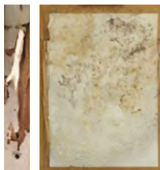
Figure 1. Side bar of a painting's strainer attacked by insects (left photo) and backing-board of a work on paper attacked by mould (right photo).
